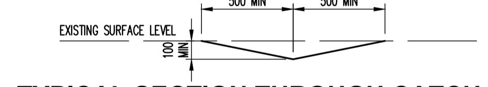
TYPICAL SECTION THROUGH CATCH DRAIN
