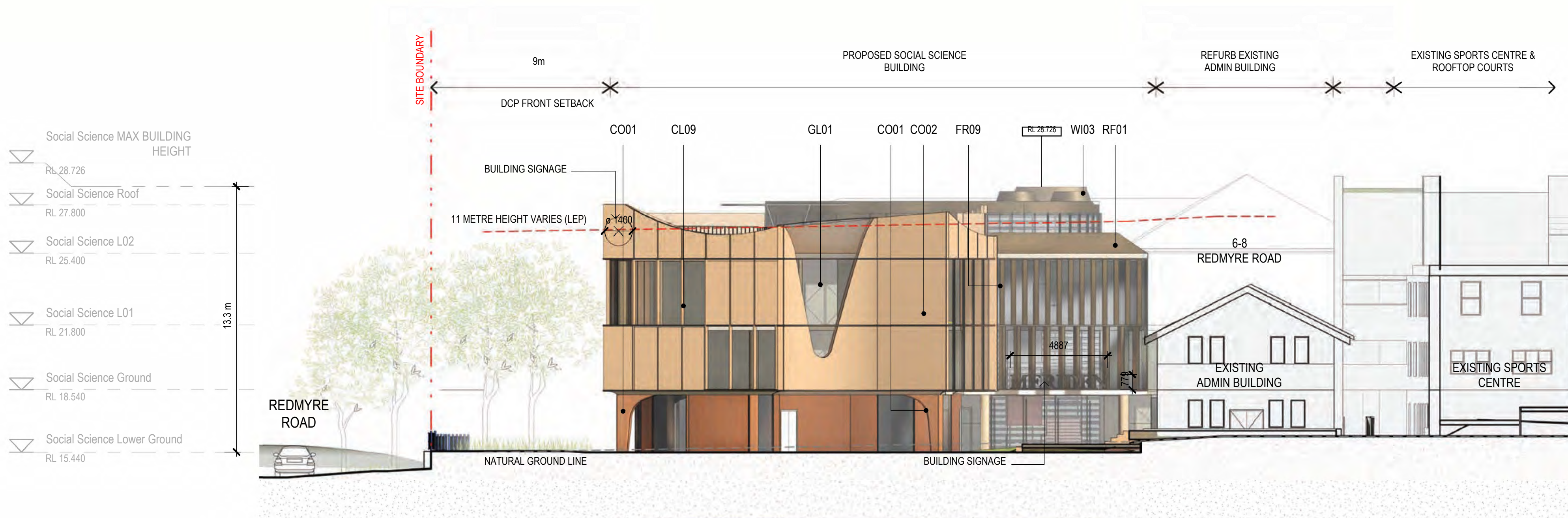
2 DA2000 - Social Science Building - West Elevation SCALE: 1 : 150
